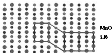
FIGURE 1 Monoclinic stacking fault (Sec Color Plate IV).
